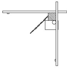
Aerial view of stud and braces. Note that the service lines extend at a 45 degree angle from within the braces
